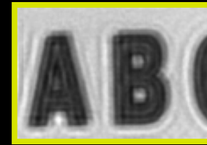
Ringing with the traditional Richardson-Lucy deconvolution algorithm
